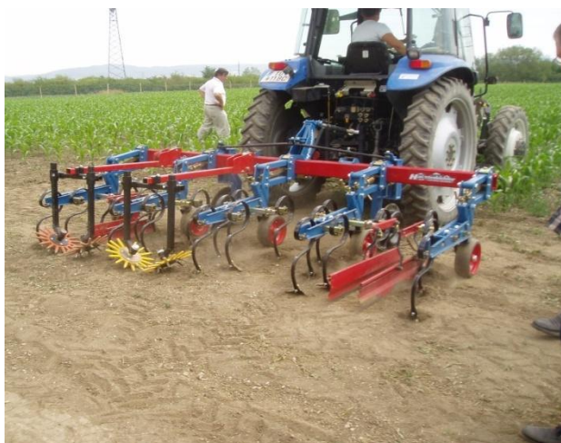
Figure 2: Test of different tool for inter row cultivator
